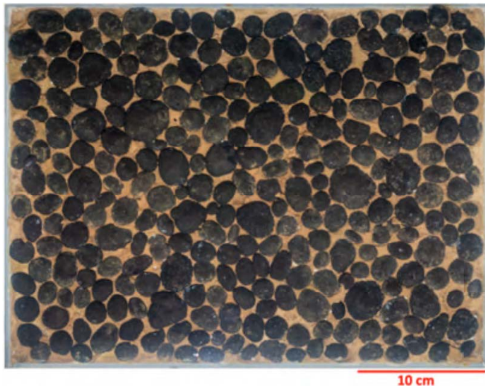
Fig.4. Test section, with 286 Type 1 nodules from the NORI exploration site ( \approx 16 kg ww)
